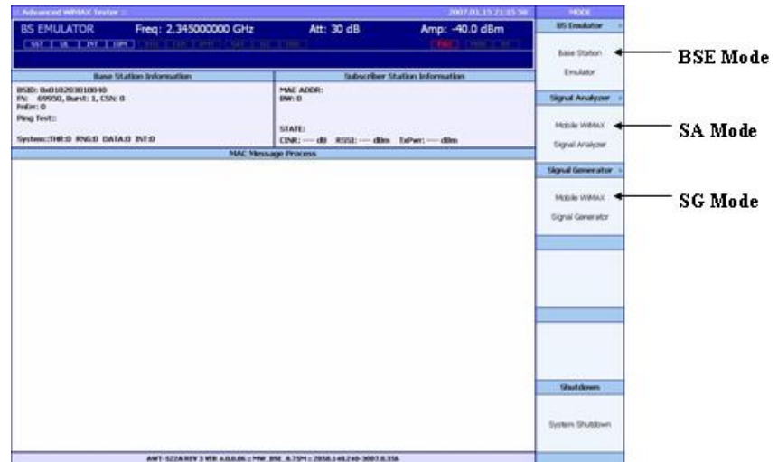
Figure 9 E6651A Test Set Operational Mode Selection Window
